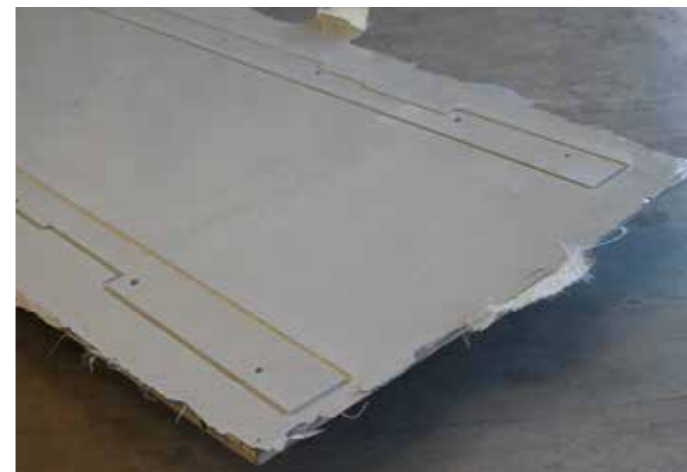
Deck section fresh out of the mould with first machining cuts made.
