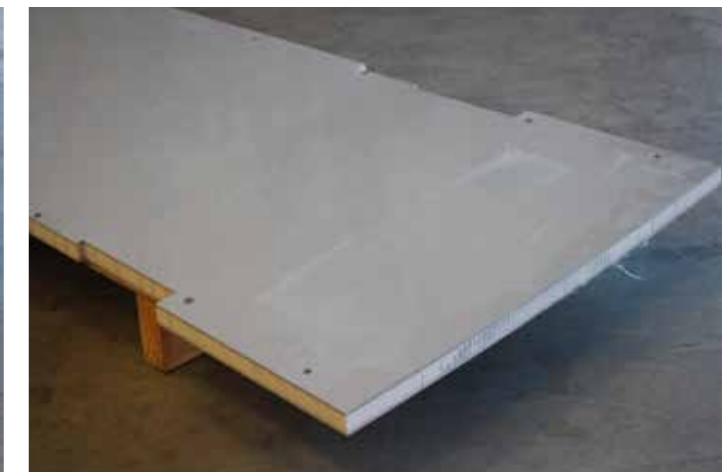
Finished machined deck section.
